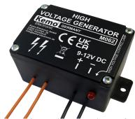
Produces from a battery voltage of 9 - 12 V/DC a pulsating, weak high-tension of approx. 1000 Volt. For electrically operated fences for small animals, as thief-protection etc. The two high voltage wires must be simultaneously connected to the bare feet, tongue, snout or other part of the small animal to induce electric shock.
